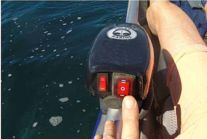
Battery connection, in a waterproof compartment
